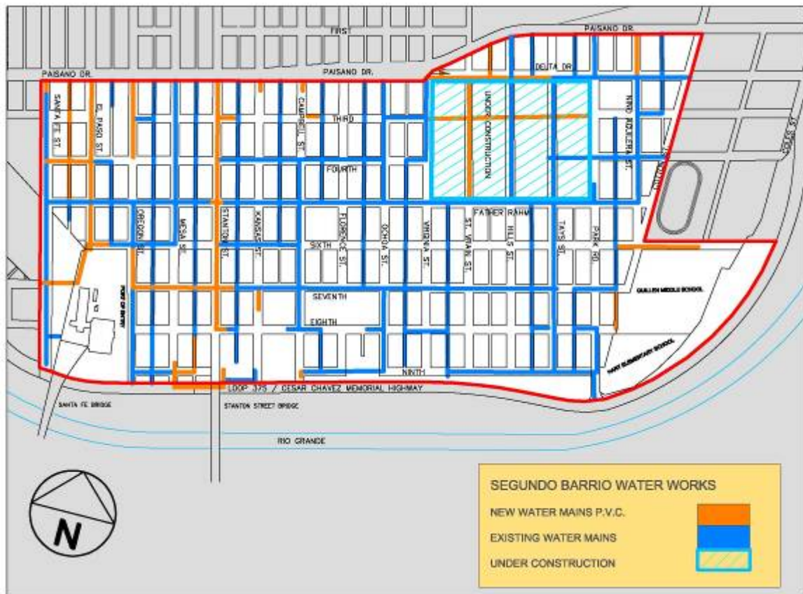
Figure 2.10: Waterline Improvements, El Paso Water Utilities 2009
