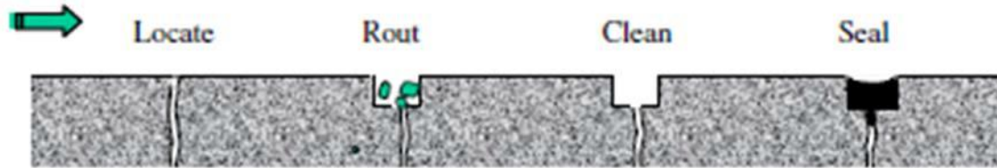
Illustration of Crack Routing, Cleaning, and Sealing
