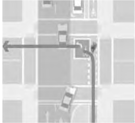
Figure C3. On separated bike lanes, the two-stage turn box can be located in the protected buffer/parking area.
