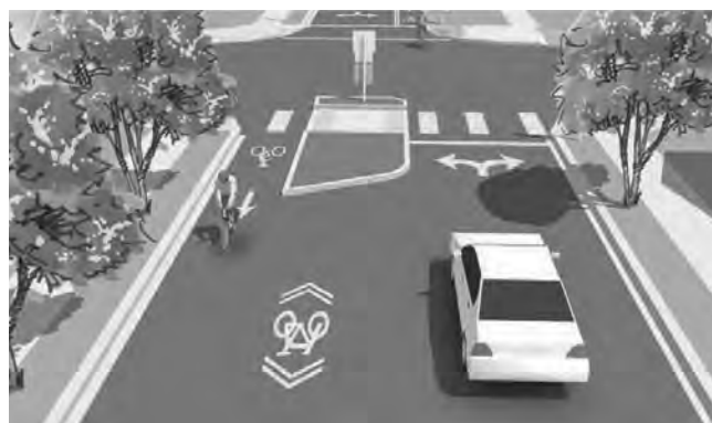
Figure C26. Traffic diverters allow through bicycle movements while restricting motor vehicle traffic.
