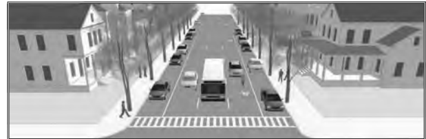
Step 1: A low cost and immediate improvement for the corridor would be the addition of Shared Use Lane Markings or "Sharrows" to indicate that this is a preferred bicycle route.
