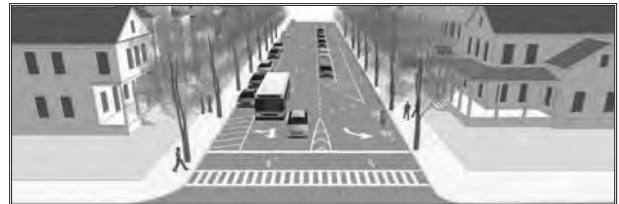
Step 3: The addition of a parking protected cycle track and bicycle box would attract a greater number of cyclists and would be appropriate on major routes.
