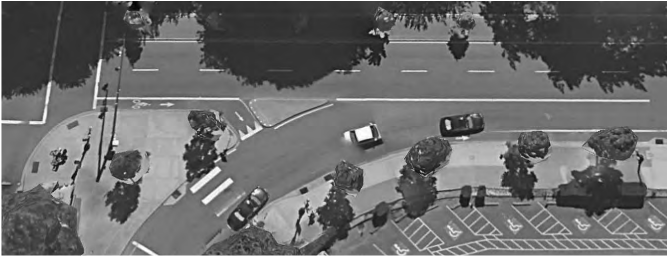
Figure C14. Bicyclists are channelized in advance of the crossing to encourage them to yield to entering motor vehicles in this example from Portland, OR.
