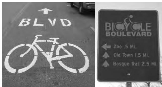
Figure C23. A combination of pavement markings and distinct signs distinguish bicycle boulevards from other shared travel lanes.
