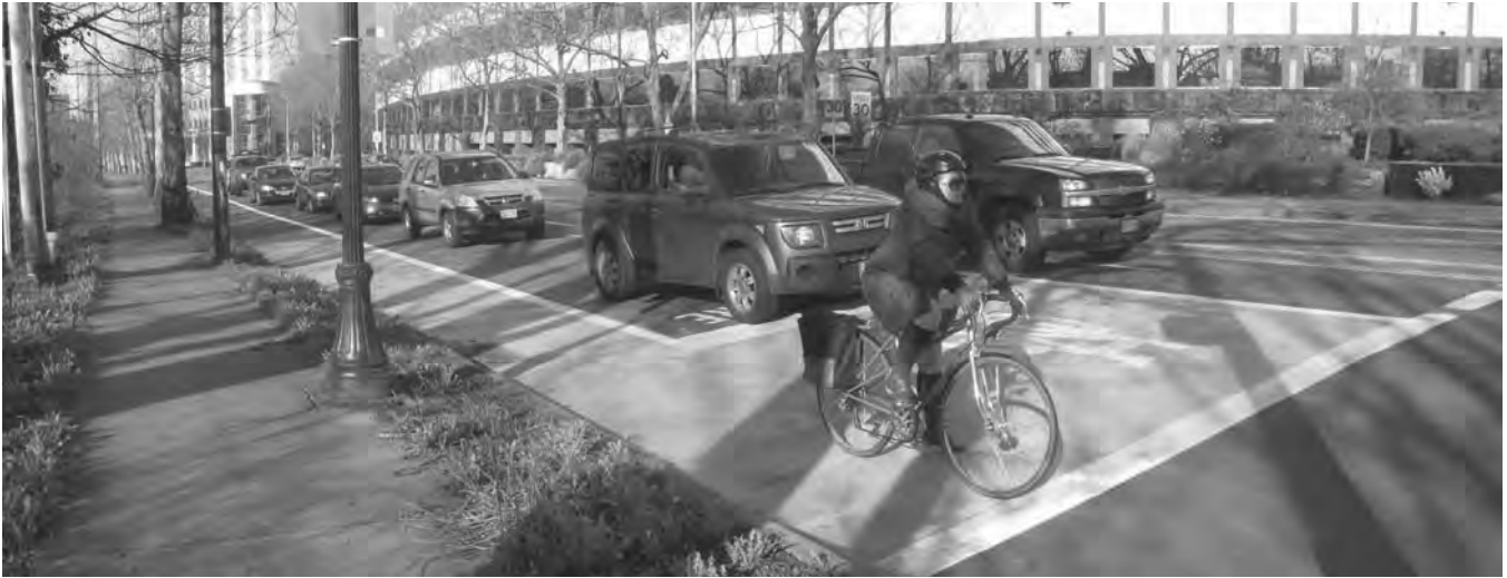
Figure C1. A bike box allows for cyclists to wait in front of queuing traffic, providing high visibility and a head start over motor vehicle traffic.
