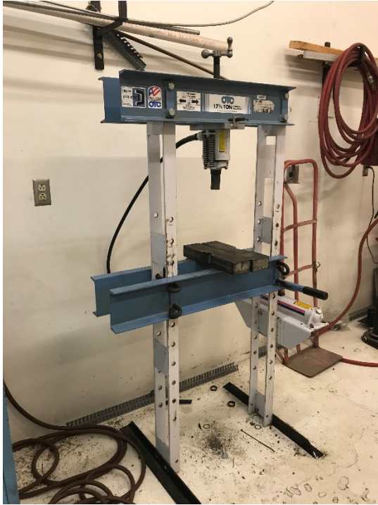
SPX OTC -HYDRAULIC PRESS 17.5 TONS- WITH HYDRAULIC PUMP MODEL B-MAX W.P. 10,000psi -LOCATED IN THE MACHINE SHOP NORTH SIDE OF THE BUILDING
