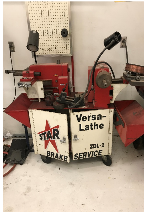
STAR BRAKE LATHE MACHINE - MODEL ZDL-2 -120V 1PH 60HZ -LOCATED INSIDE THE MACHINE SHOP NORTHSIDE BUILDING
