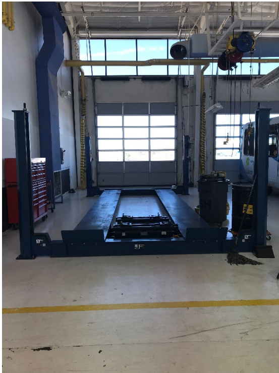
THREE ROTARY 4 POST LIFTS- MODEL SM300-200- 30,000LBS CAPACITY EACH LIFT- 208V 3PH 60HZ- TWO LIFTS WERE INSTALLED IN 2001 AND ONE LIFT WAS INSTALLED IN 2018
