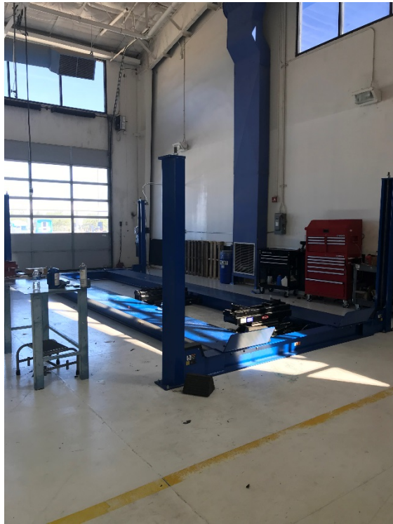
THREE ROTARY 4 POST LIFTS- MODEL SM300-200- 30,000LBS CAPACITY EACH LIFT- 208V 3PH 60HZ- TWO LIFTS WERE INSTALLED IN 2001 AND ONE LIFT WAS INSTALLED IN 2018
