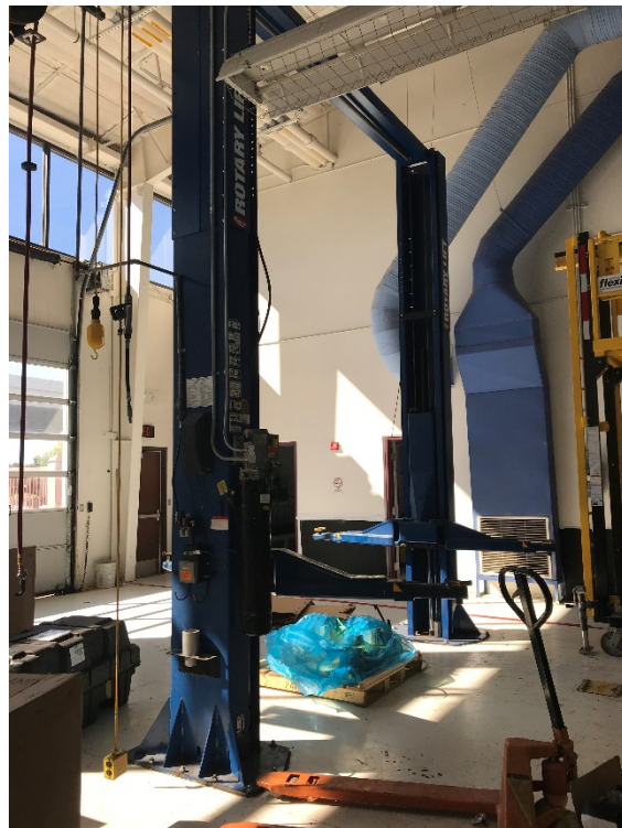
THREE ROTARY 2 POST LIFTS- MODEL SPO18N210 18,000lbs CAPACITY -208V 3PH 60HZ-ALL THREE INSTALLED IN 2001. EQUIPMENT LOCATED IN THE MAINTENANCE SHOP
