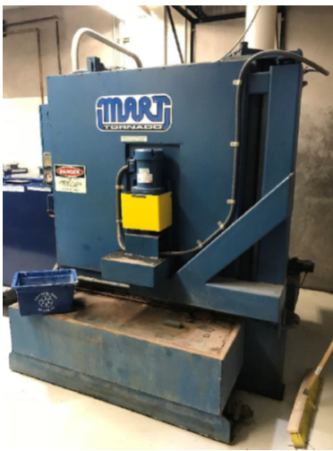
MART AUTOMOTIVE POWER WASHER – TORNADO 40- 460 VOLTAGE 60HZ 3PH - YEAR INSTALLED 2001. POWER WASHER IS NOT IN USE-INSIDE OF CABINET IS RUSTED AND IS BEYOND REPAIR. LOCATED INSIDE COMPRESSOR RM ON NORTHSIDE OF BUILDING
