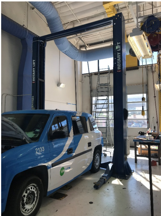
THREE ROTARY 2 POST LIFTS- MODEL SPO18N210 18,000lbs CAPACITY -208V 3PH 60HZ-ALL THREE INSTALLED IN 2001. EQUIPMENT LOCATED IN THE MAINTENANCE SHOP
