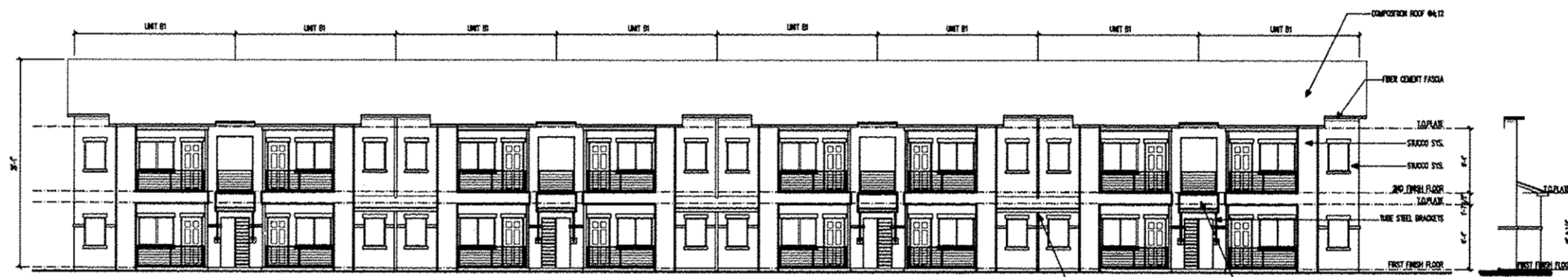
FRONT ELEVATION BUILDING TYPE III SCALE 1/8"=1'-0" STUCO 1/8"
